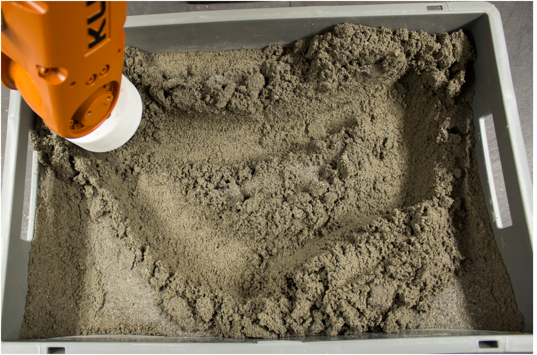
Figure 35: A curve can be deduced in the bottom of the picture with a connecting line in the top, which is due to the repetition of the movement. Through experimenting with parameters, we unexpectedly came up with The Dented Curve .
