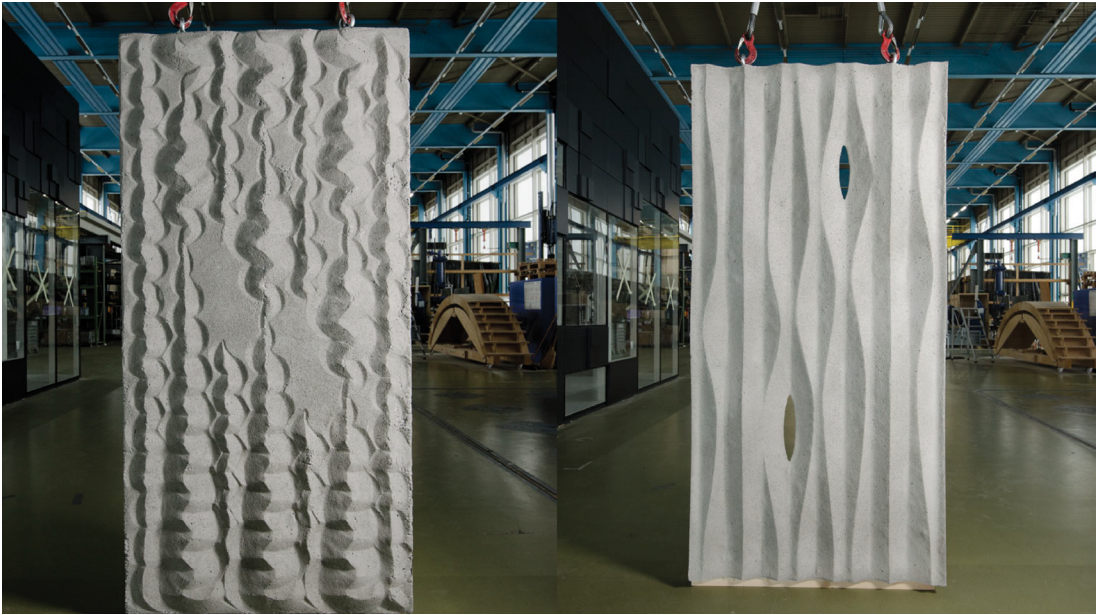
Figure 7: The finalized pre-fabricated concrete wall blocks that was created through intricate molds based on shapes drawn in sand (Gramazio Kohler Research, 2011 - Procedural Landscapes 2)
