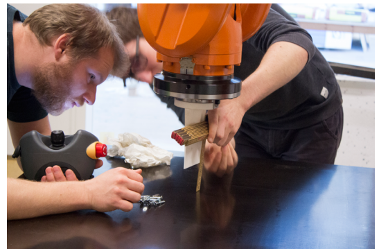
Figure 11: Students measuring the distance between the end-effector and the surface, which is used to offset the toolpath in the software.
