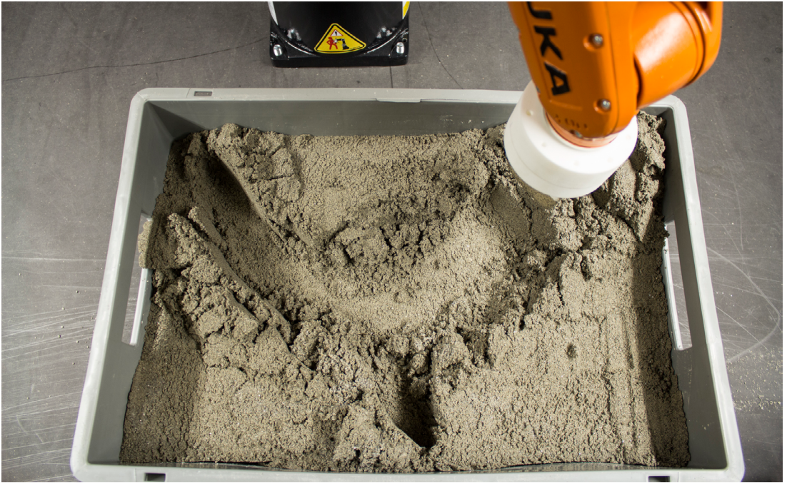
Figure 29: A top view of the sandbox after experimenting with a keyboard for controlling the robot. An error can be seen in the bottom, where the end-effector goes too far.
