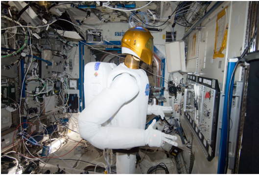
Figure 3: Robonaut 2 onboard the International Space Station. Teleoperators can interact, through the Robonaut, with equipment and onboard astronauts or kosmonauts. (NASA, 2013)
