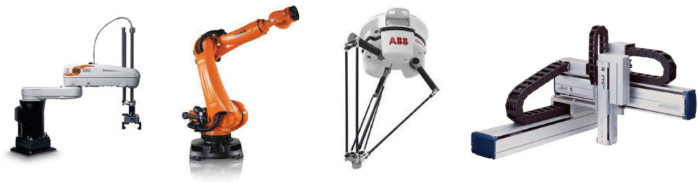
Figure 5: Types of Robots - From left to right: SCARA, Articulated, Parallel and Cartesian Robot (KUKA Robotics, 2006 - SCARA) (KUKA Robotics, 2015 - Quantec) (ABB, 2013) (Toshiba Machine Company, 2015).
