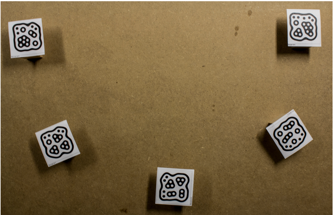
Figure 36: The toolpath starts with the upper-left blocks and goes sequentially to the upper-right block. Notice the differing orientation of the markers, causing the end-effector to rotate during execution.
