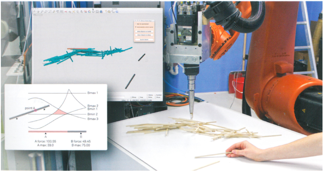
Figure 9: The human provides the robotic agent with wooden sticks and determines how it should be placed by orienting it. The robotic agent then decides where to put it on the existing structure, based on the architect's chosen orientation and where it maintain most stability.
