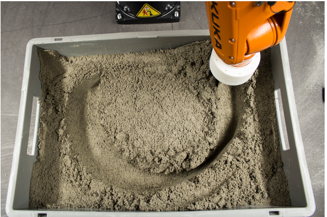
Figure 34: Using three blocks, an almost perfect curve has been created. This was done iteratively, adjusting the positioning of the blocks. The variable stroke is caused by the constant orientation of the spatula.
