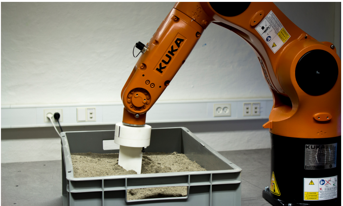
Figure 28: The spatula, which was 3D printed on an EOS Formiga 3D printer (EOS, 2013), has been mounted on the mounting flange of the sixth axis of the robot. The image showcases our testing of the structural strength of the spatula in granite sand.
