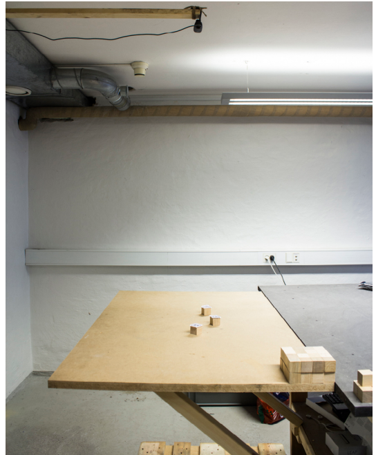
Figure 24: The tangible user interface setup on a surface for placing blocks. These blocks are tracked by the webcam mounted above
