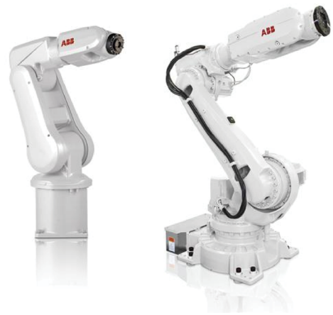
Figure 10: The ABB IRB120 (Left) and the ABB IRB6620 (Right) Articulated arms. The ABB IRB120 has a reach of 58 centimeters, compared to the ABB IRB6620's reach of 2,2 meters (ABB,2015 - IRB120 and IRB6620). The picture does not depict relative sizes.
