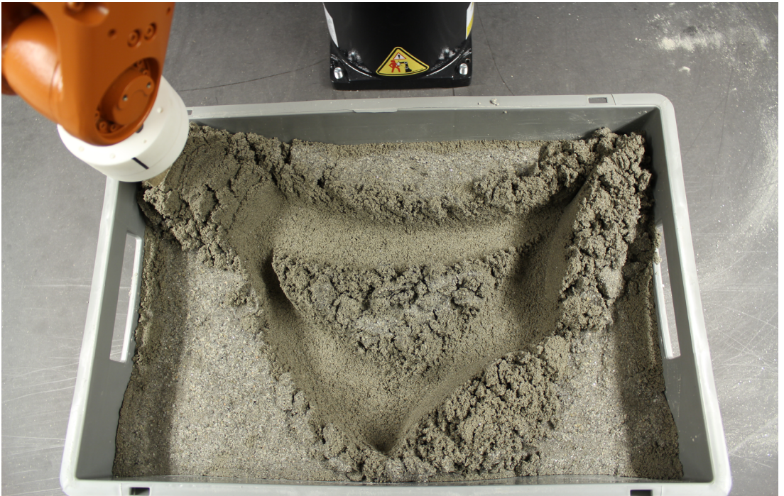
Figure 33: This curved triangle was caused by the repeated toolpath movement of the robot, using blocks for controlling X, Y and yaw.
