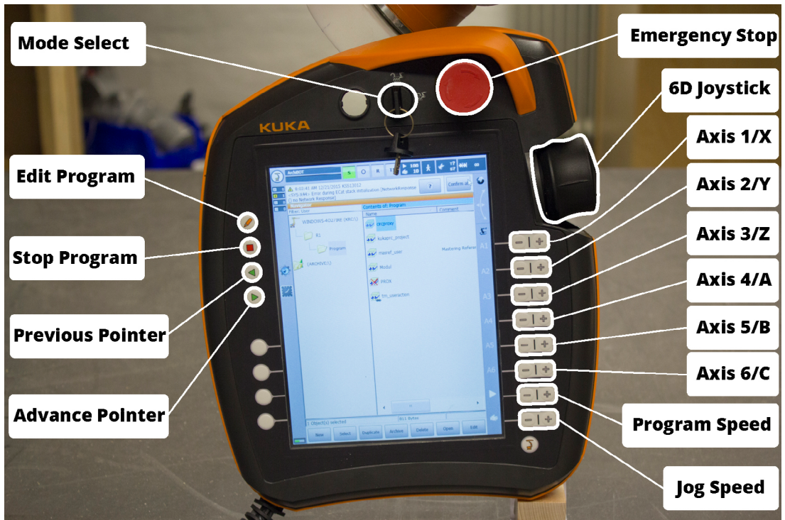
Figure 6: The KUKA SmartPad running KUKA's own software for configuring the controller and robot. The SmartPad has a touchscreen, physical buttons and a six dimensional joystick for jogging the robot.
