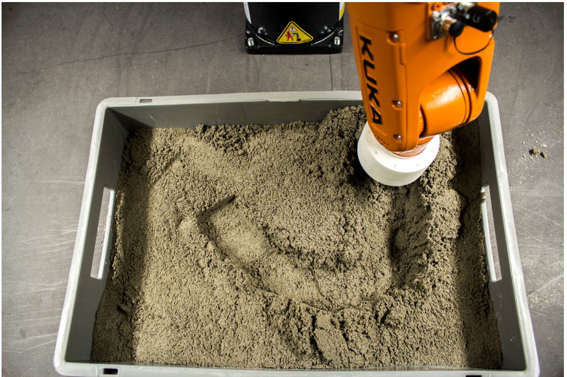
Figure 32: The above result is caused by the rotation of the interacting hand being mapped to yaw causing a straight stroke throughout the curve.
