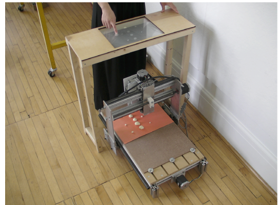
Figure 6: Prototype of 3D printer interface. The user can do a real-time manipulation of the printed object (Willis, et al. , 2011).
