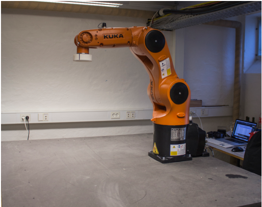
Figure 9: The KR6 R700 sixx robot mounted on a 25 mm black MDF tabletop.
